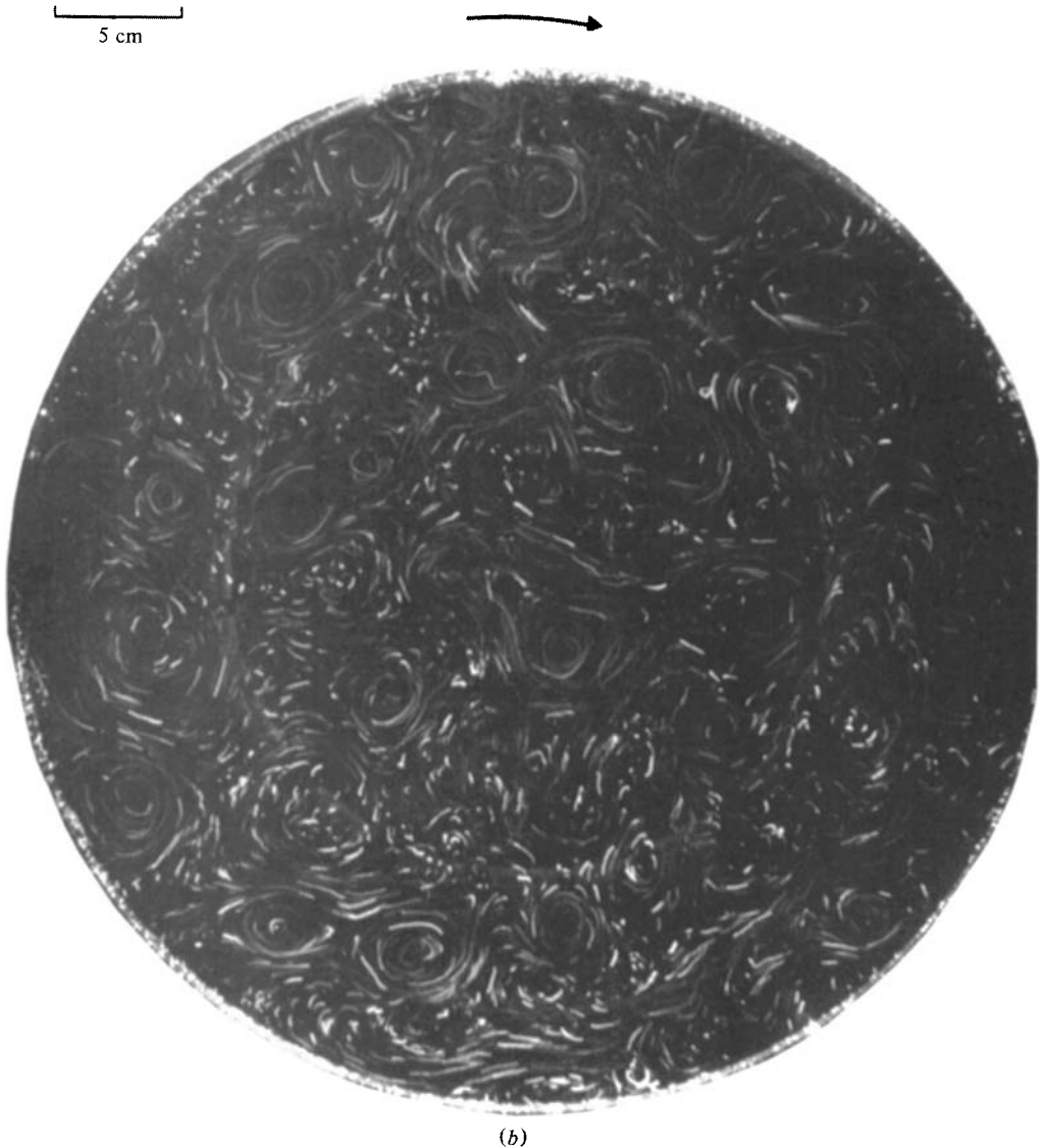
FIGURE 2. Streakline photographs of the turbulent flow field in a cross-section of the tank 30 cm above the grid midplane, (view from above): (a) without rotation, n = 13.3\pi \text{ rad s}^{-1} , ( S = 4 \text{ cm} ); (b) with rotation (clockwise tank rotation as indicated by the arrow), n = 13.3\pi \text{ rad s}^{-1} , \Omega = 2\pi \text{ rad s}^{-1} ( Ro_g = 3.32 ). The exposure time was 0.25 s.
